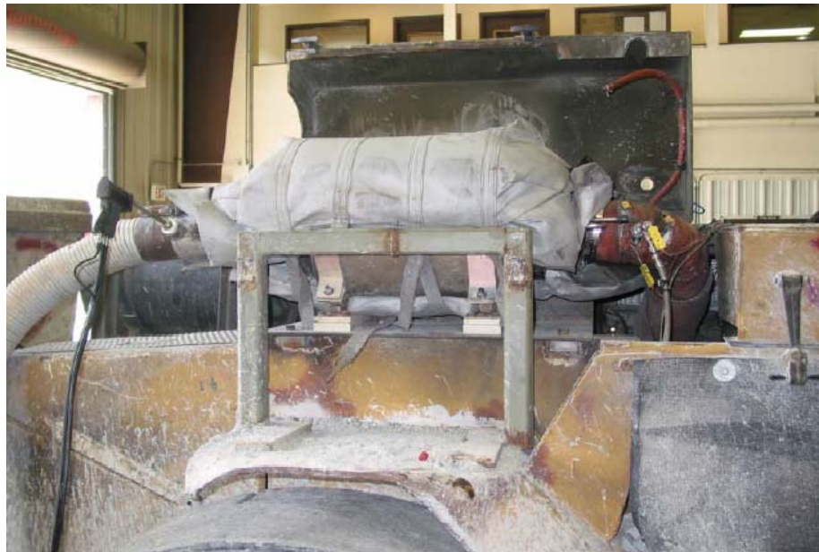
Figure 2: Pt Catalyzed Cordierite DPF Installed on Truck
