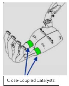
Figure 9. Advanced motorcycle exhaust system including close-coupled catalysts<sup>4</sup>.
