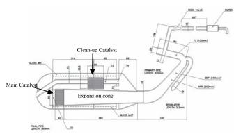
Figure 7. Two-stroke 50 cc moped muffler equipped with SAI via reed valve and dual catalysts, in separate locations to control exhaust temperature.
