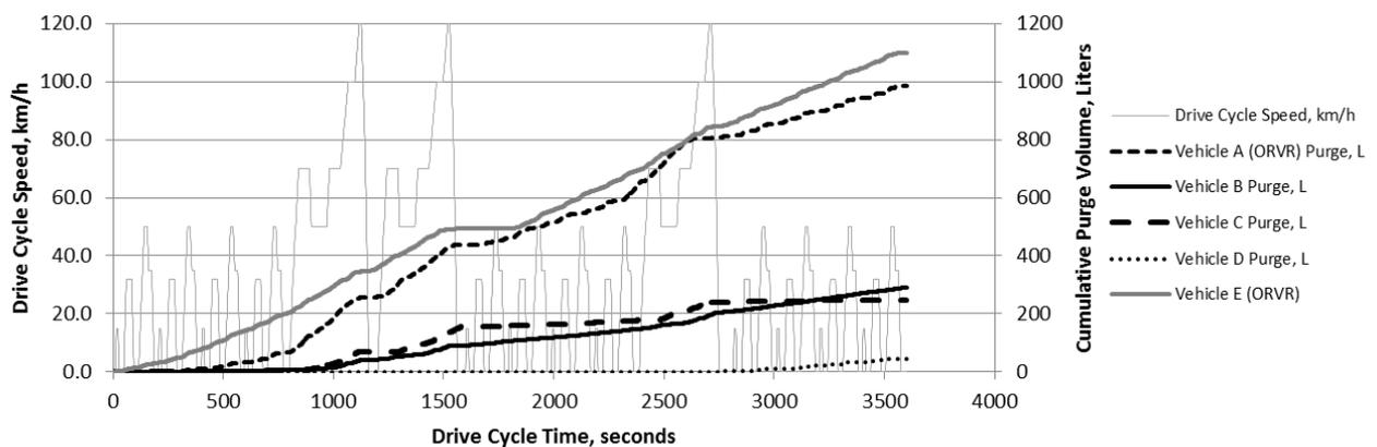
Figure 3. Canister purge traces for Vehicles A, B, C, D, and E showing cumulative purge volumes over the NEDC. The ORVR-equipped Vehicles A and E ingested over 1,000 liters of purge air, while Vehicles B and C ingested 250-290 liters. Vehicle D only ingested 50 liters of purge air. Note that the majority of purge occurred during the highway section of the NEDC. Vehicles B, C, and D purged very little over the low-speed urban portion of the NEDC.
