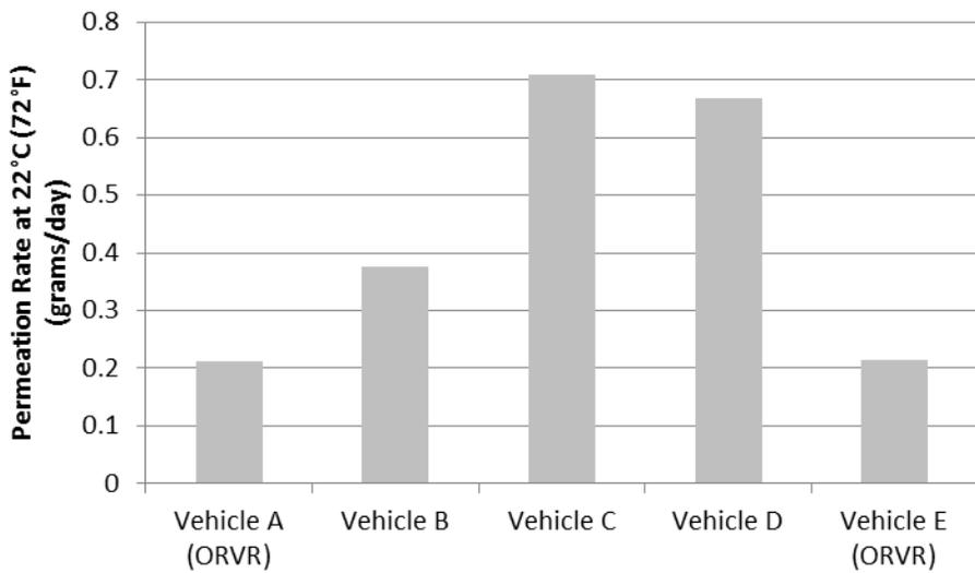
Figure 7. Permeation rates for Vehicle A, B, C, D, and E measured by venting the canister outside of a SHED held constant at 22°C (72°F) for 24-hours. Permeation rates for Vehicles B, C, and D were 2-3 times higher than that of Vehicles A and E that utilize low permeation materials.
