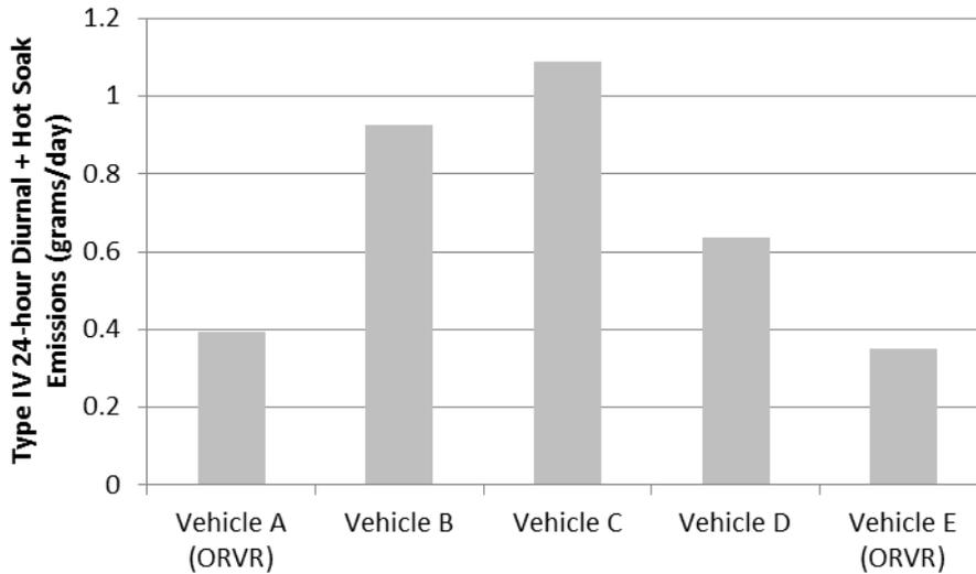
Figure 2. SHED diurnal emissions for Vehicles A, B, C, D, and E following the Chinese Type IV 24-hour diurnal procedures, which has a 2 g/day limit. All vehicles met this requirement, but the ORVR-equipped Vehicles A and E produced half the emissions of the non-ORVR vehicles.
