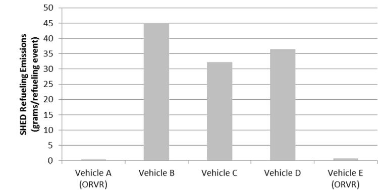
Figure 1. SHED refueling emissions measured for Vehicles A, B, C, D, and E at Beijing CATARC. Vehicles A and E were equipped with ORVR, which provided >99% control of refueling emission (note refueling emissions for vehicle A and E were only 0.5 grams)
