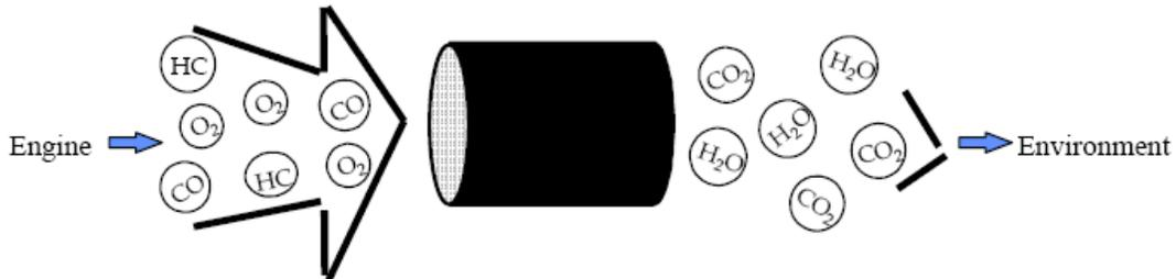
**Figure 5. Diagram of two-way oxidation catalyst showing reactants and products in the exhaust.**
