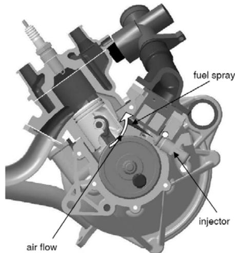
**Figure 1. Schematic of a two-stroke engine fitted with low pressure fuel injection (SAE 2006-32-0065).**
