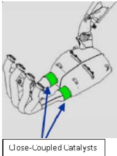
**Figure 9. Advanced motorcycle exhaust system including close-coupled catalysts<sup>4</sup>.**
