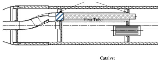
**Figure 8. Catalyzed heat tube attached to muffler intake facilitates exhaust light-off.**
