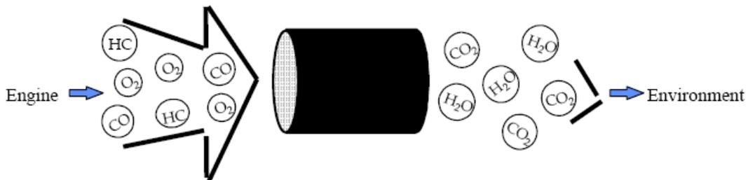
**Figure 5. Diagram of two-way oxidation catalyst showing reactants and products in the exhaust.**
