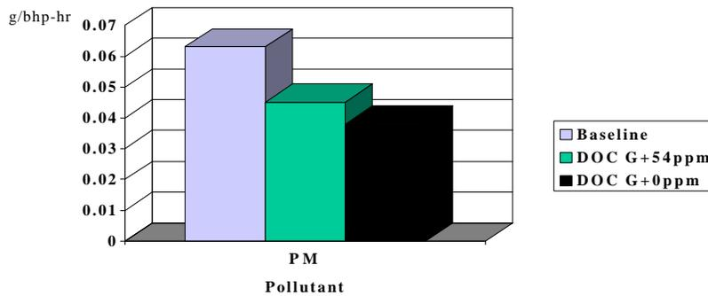
The zero sulfur fuel enabled the catalyst to reduce PM emissions from 0.045 g/bhp-hr when tested with 54 ppm sulfur fuel to 0.038 g/bhp-hr when tested with it.
