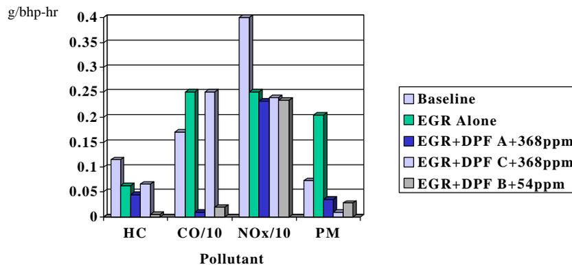
The results of the testing indicate that the combination of DPF technology and EGR achieves simultaneous NOx + HC emissions of less than 2.5 g/bhp-hr and PM emissions of less than 0.05 g/bhp-hr on both fuel containing 368 ppm and 54 ppm sulfur.
