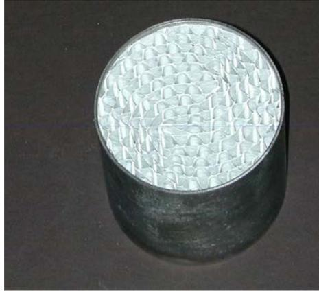
Figure 11: Zeolite based AIS hydrocarbon trap
