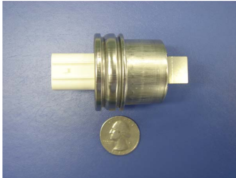
Figure 18. Onboard urea quality sensor.
