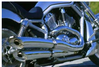
Figure 4. Catalyst engineered and integrated to fit inside the chrome muffler.
