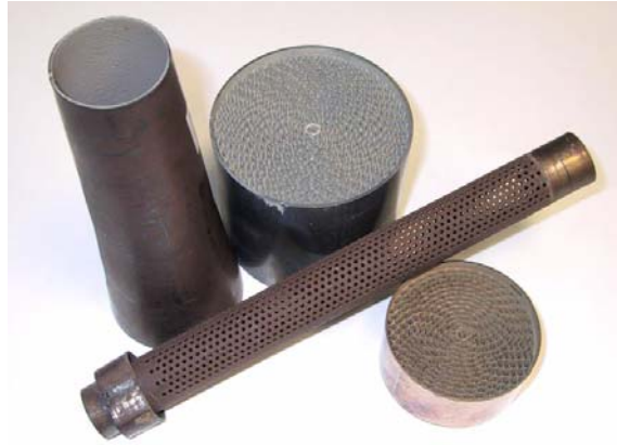
Figure 3. Motorcycle catalysts and substrates can take on many shapes and sizes. These may include coated expansion cones, perforated heat tubes, and coated metallic substrates.
